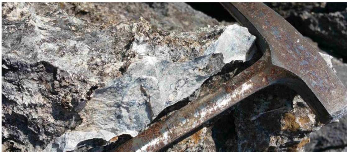
Figure 4 – Outcropping disseminated galena (dark grey) and sphalerite (brown-grey) mineralisation with secondary zinc oxides (brown) in the Auros area.
